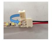
5. For end connection or jumping open one side of the connector and slide the end of the tape until it is flush with the back of the connector as shown. Close the connector top and snap in place. Make sure the (+) dot lines up with the red wire.
