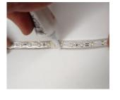
8. Splice connectors are available for joining cut pieces and each side should be installed following steps 3-5. Make sure to alight the (+) dot to the (+) dot on each corresponding side of the splice connector.
